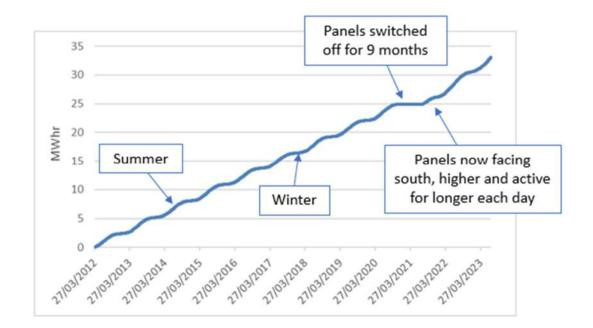
The following graph shows the total generated power of our system since installation:
